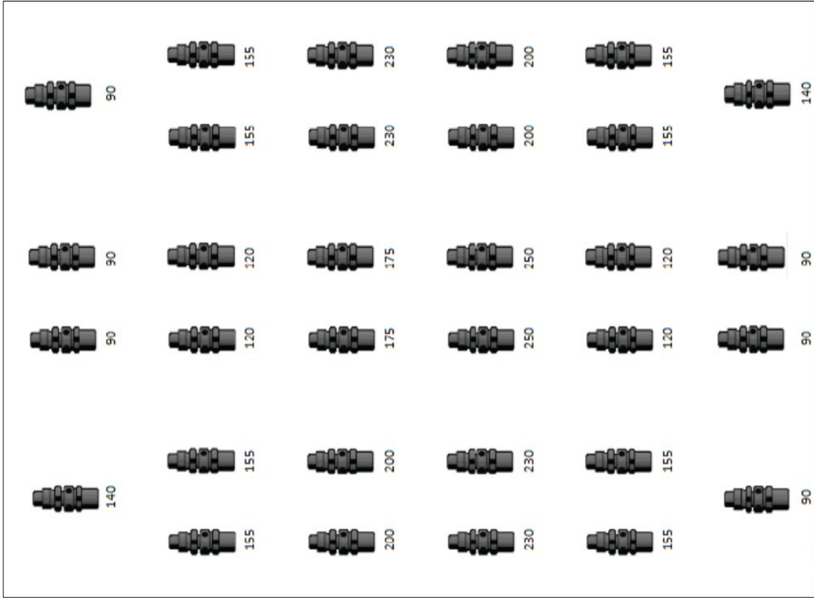
Figure 3. Source array configuration for the proposed ocean bottom node (OBN) and distributed acoustic sensing (DAS) survey.
