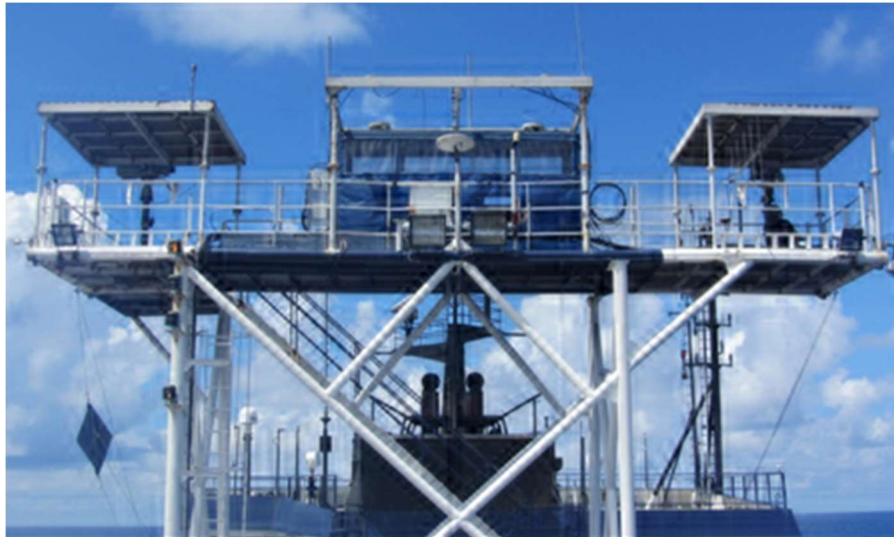
Figure 2: Protected Species Observer stern view of observation tower with mounted big-eye binoculars.
