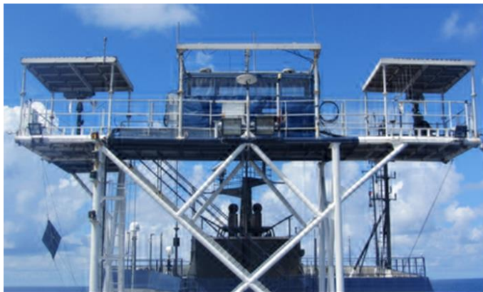
Figure 5: Protected Species Observer stern view of observation tower with mounted big-eye binoculars.
