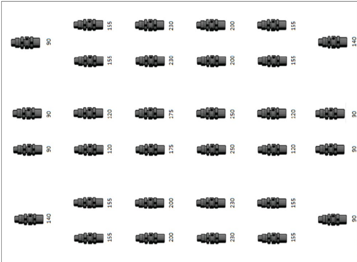
Figure 2. Source array configuration for the proposed ocean bottom node (OBN) and distributed acoustic sensing (DAS) survey.
