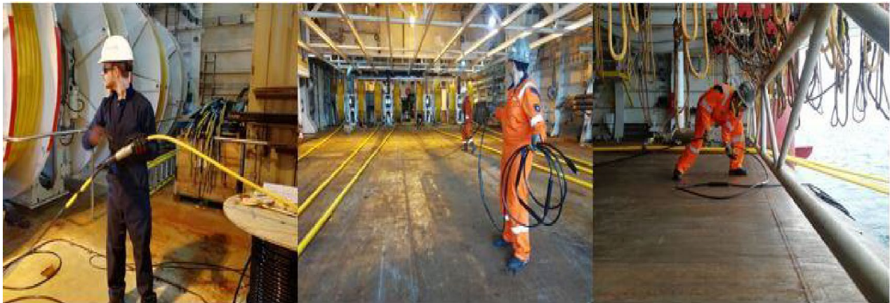
Figure 3. PAM operators manually feeding tow cable into the gun deck. Left: PAM operator directing the cable. Middle: PAM operator placing the cable on deck. Right: PAM operator manually deploying the first 3-5 meters of the hydrophone cable.
