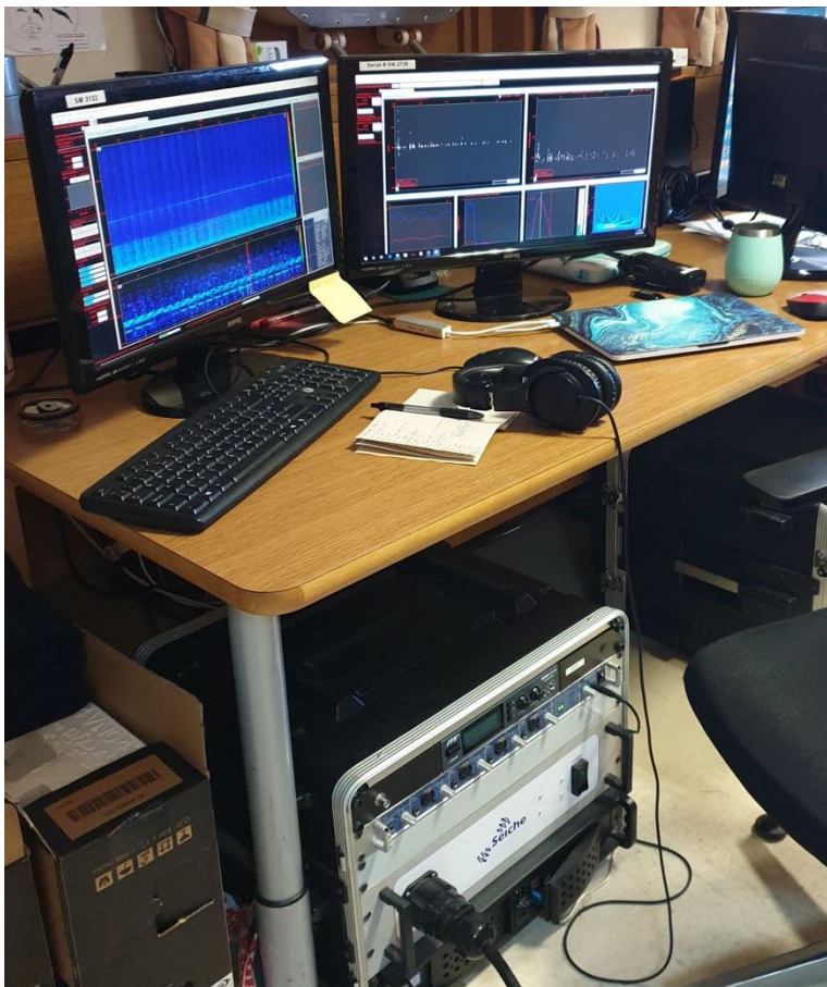
Figure 8: Passive acoustic monitoring station in instrument room.
