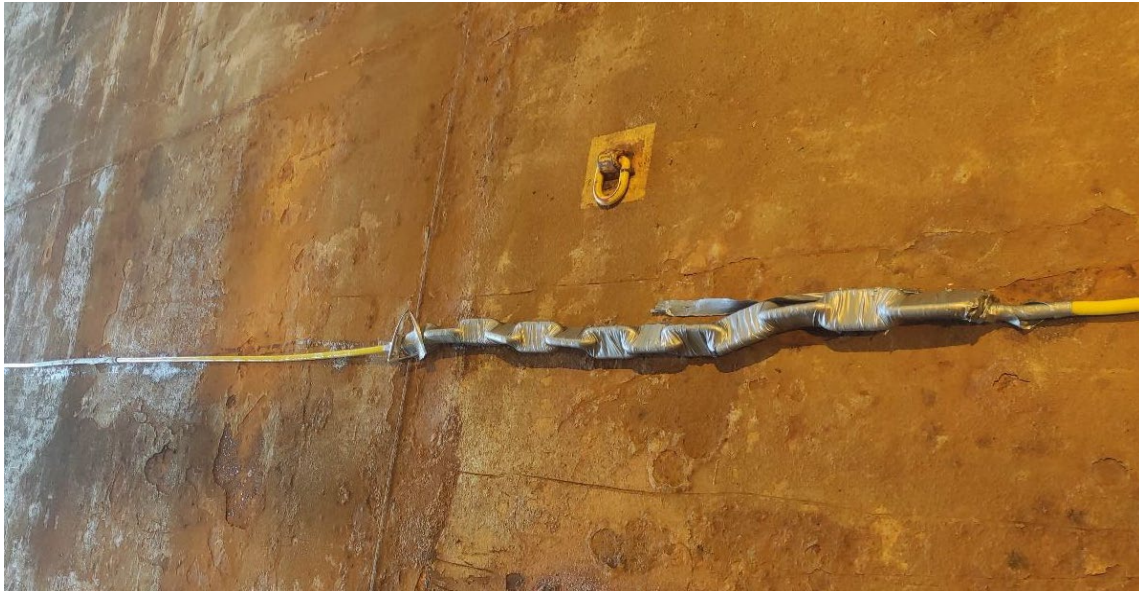
Figure 6: 5kg weight chain added to the tow cable.
