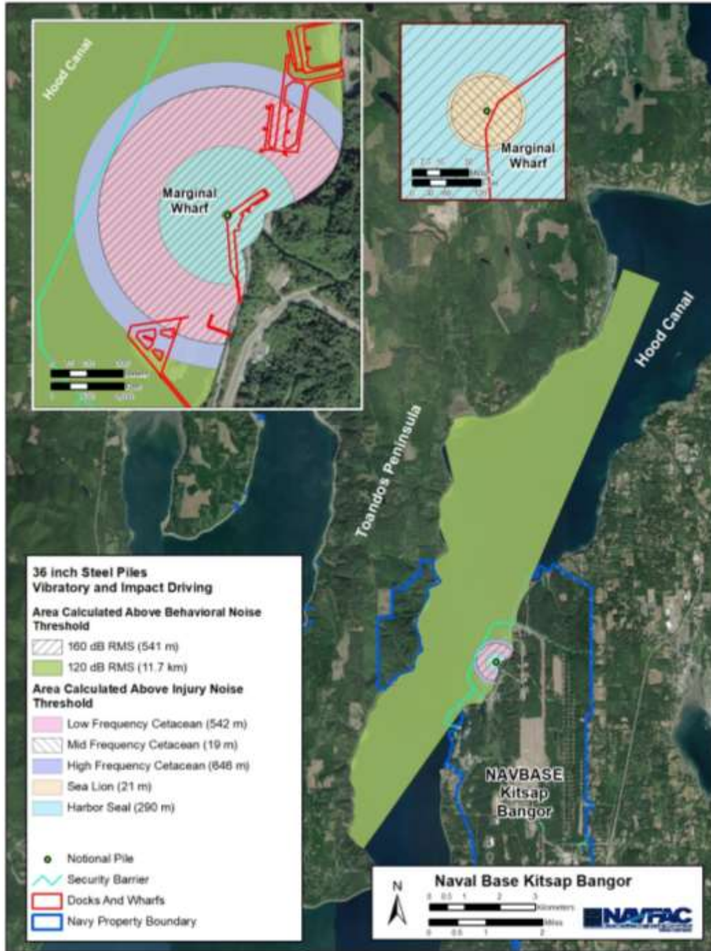
Figure 2-7. Representative Zones of Influence for Pile Driving Noise at NAVBASE Kitsap Bangor Marginal Wharf For Installation of 36 in Steel Piles (Vibratory and Impact) During the Period of July 2025 to July 2026
