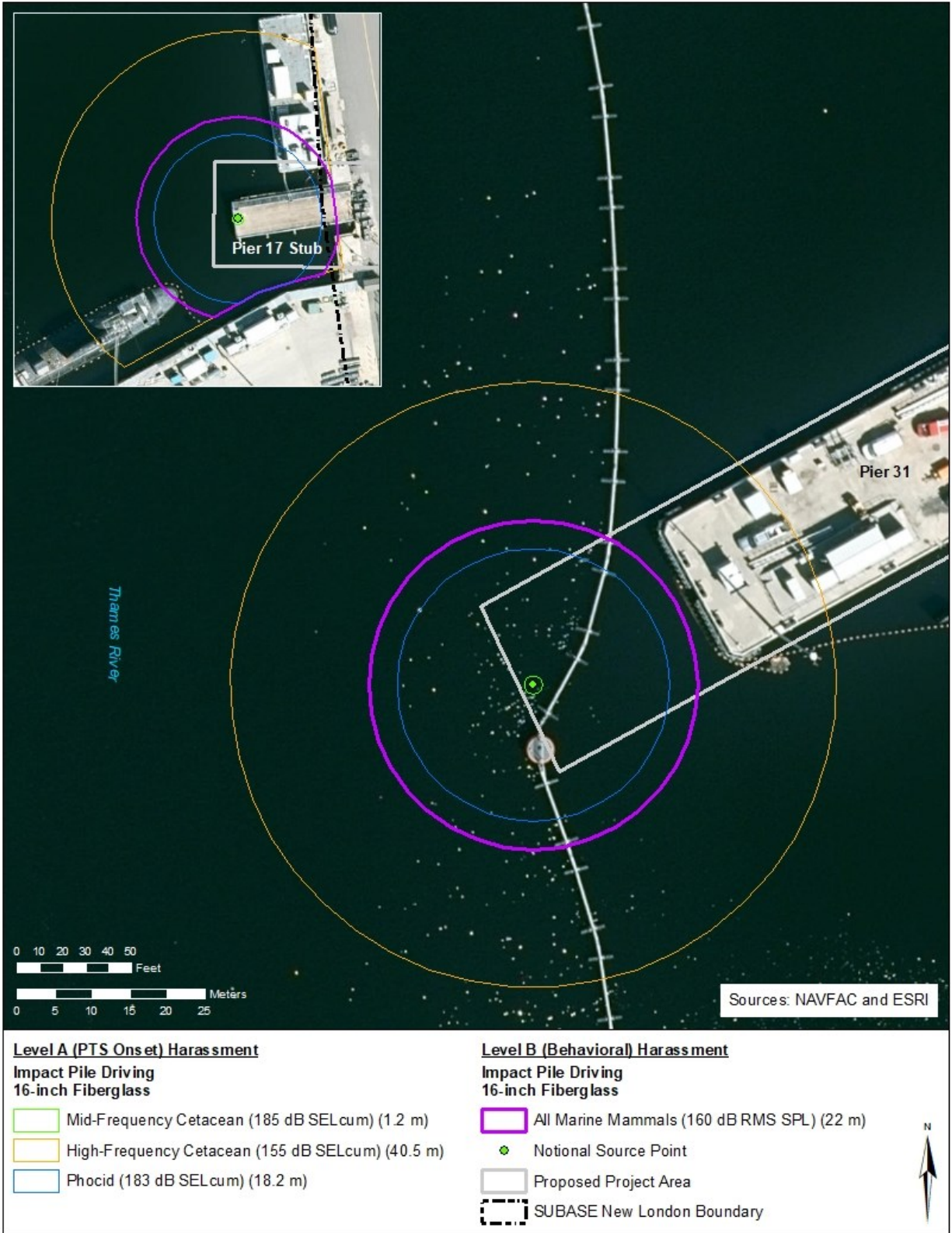
Figure 6-3 Level A (PTS Onset) and Level B (Behavioral) Harassment Zones from Impact Pile Driving – 16-inch Fiberglass Fender Piles at Pier 31 and Pier 17 Stub Quaywall
