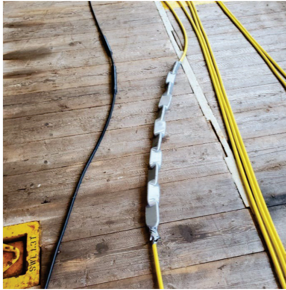
Figure 5: Chains added to the tow cable to increase depth.
