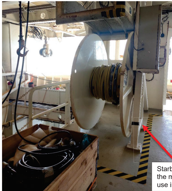
Figure 3. Hydrophone and tow cables mounted on the starboard stern winch.
