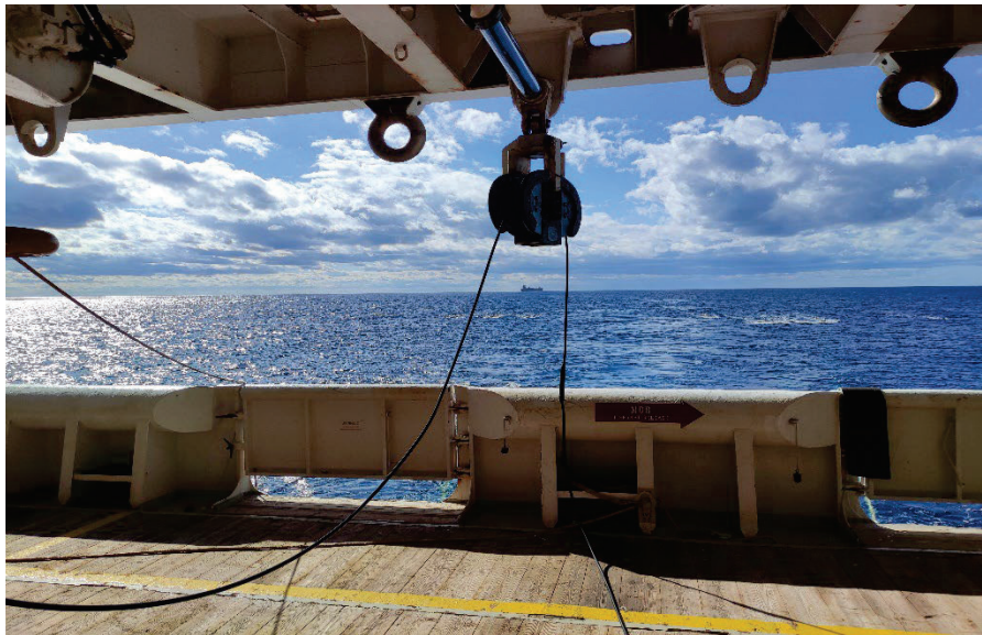
Figure 4: Cable guided through a fairlead block to the starboard stern of the vessel.
