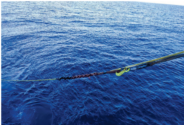
Figure 6: PAM cable fully deployed off the stern on the streamer deck.
