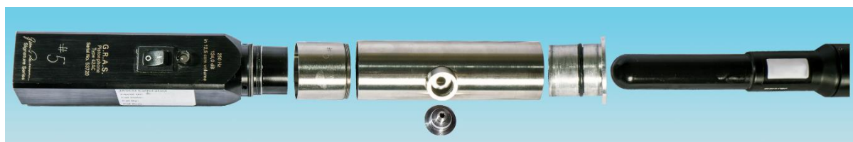
Figure E-6. Split view of a G.R.A.S. 42AC pistonphone calibrator with an M36 hydrophone.
