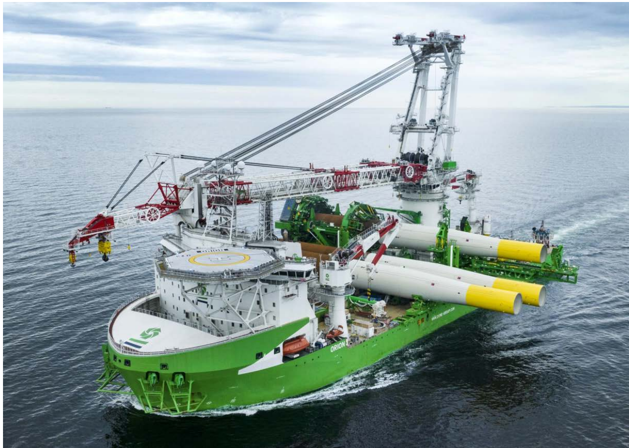
Figure 3. Monopile installation vessel (HLV Orion, 2023).
