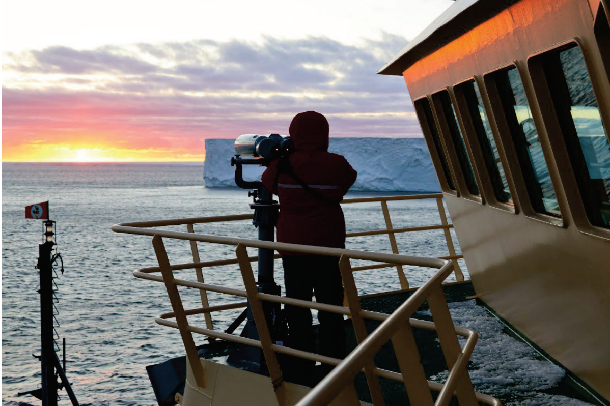
Figure 3: Big Eye binoculars mounted on the starboard bridge wing of the vessel.
