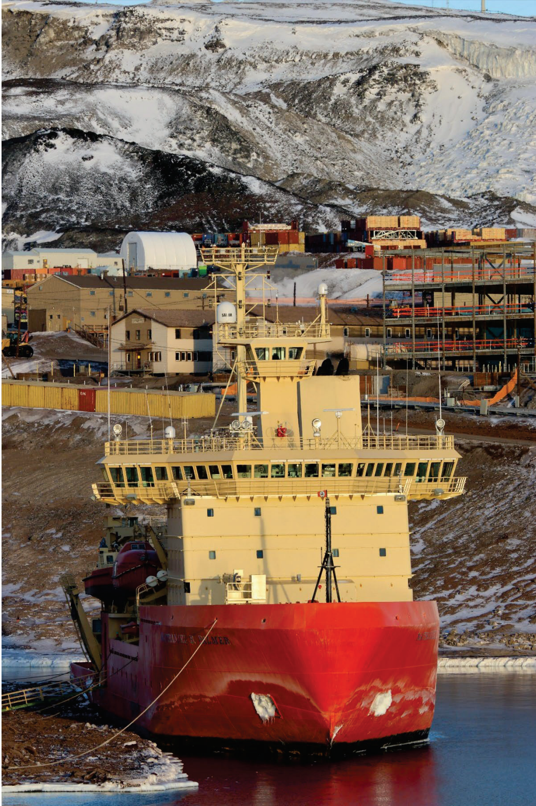
Figure 2: Front view of the NBP showing the extended bridge and bridge deck, and the ice tower above the bridge.
