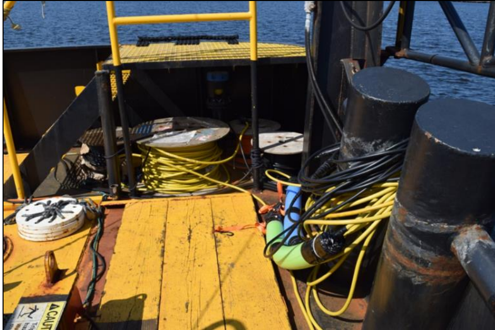
Figure E- 2: Deck and tow cable reels secured on the port stern of the vessel
