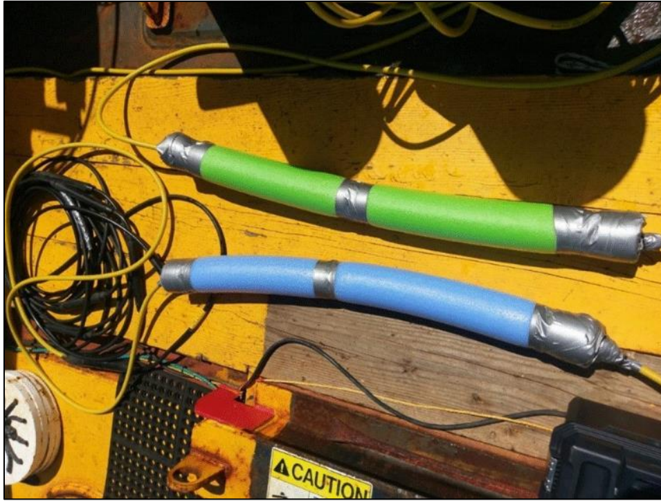
Figure E- 4: Floating tubes attached and secured to the hydrophone cable
