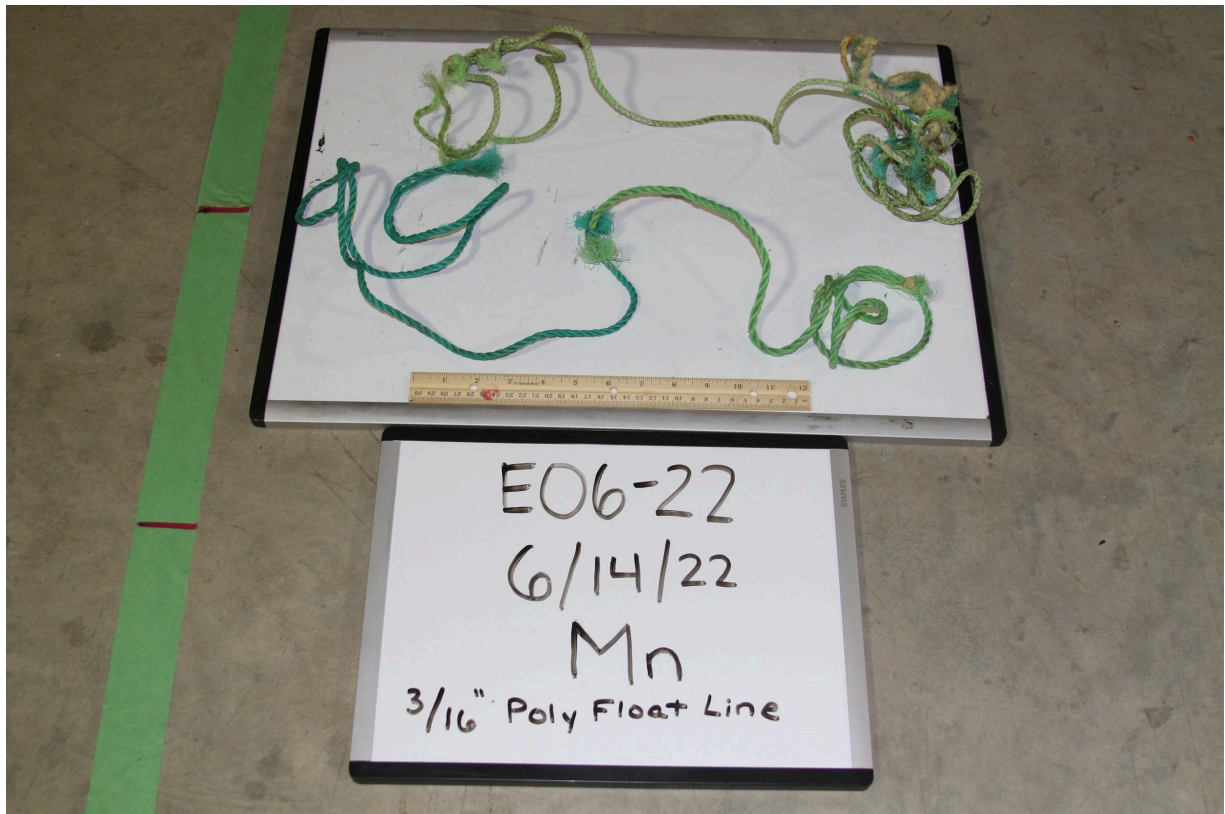
Photo 5: Small portion of recovered 3/16" rope.
