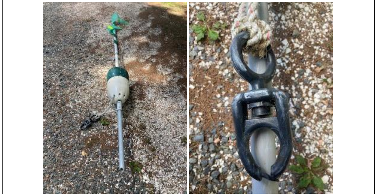
Photo 1: High flyer buoy with 600# broken weak link.
