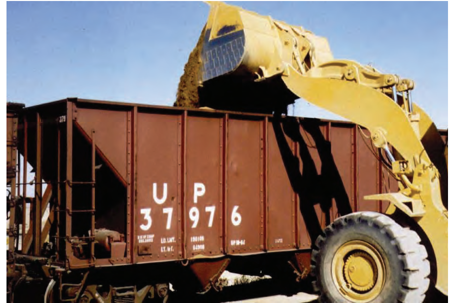
Photo B. Loader filling a bottom dump rail car
