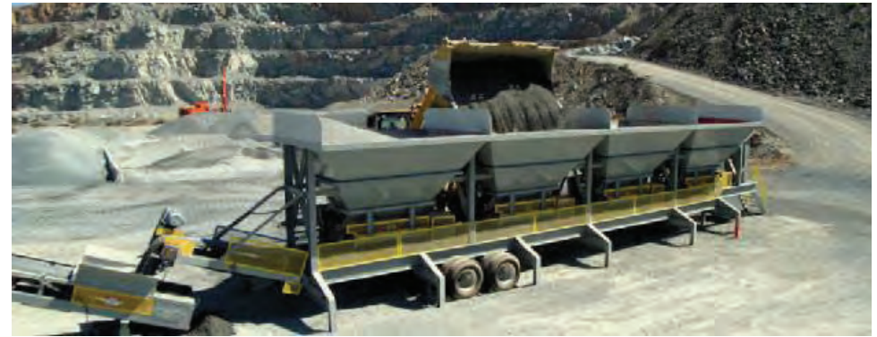
Photo D. Typical Conveyor Loading Hopper M&N Study Report for Occidental de Colombia 2012
