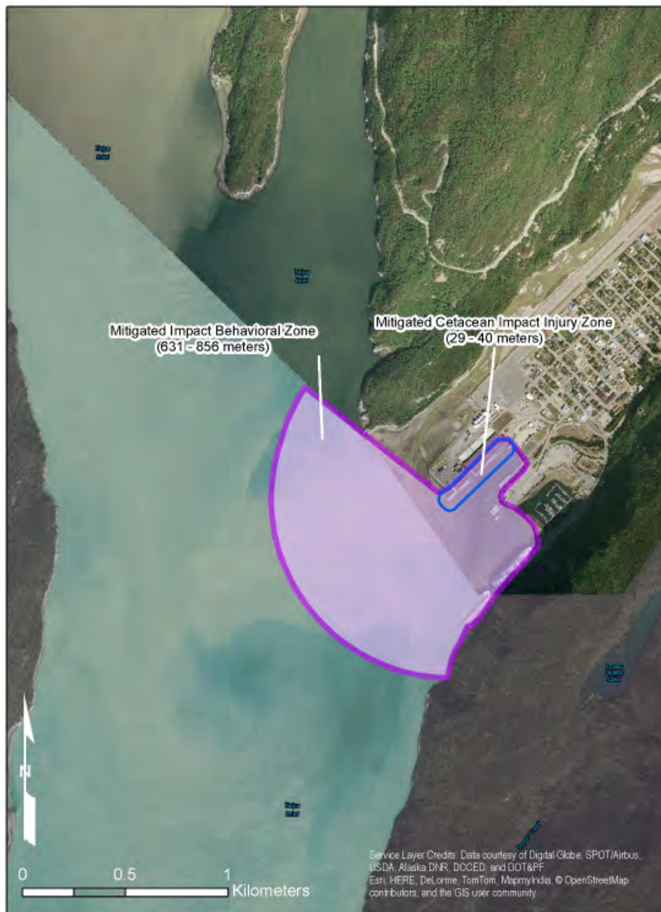
Figure 3 – Marine mammal impact pile driving behavioral and injury zones using a bubble curtain (mitigated)
